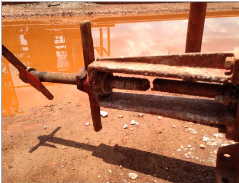
Figure 7. Broken stem in #3 DBO Pump Discharge Valve after removal (View #2)
