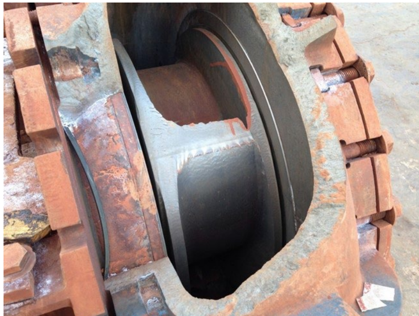
Figure 12. #3 DBO Pump failed casing close up (different angle)
